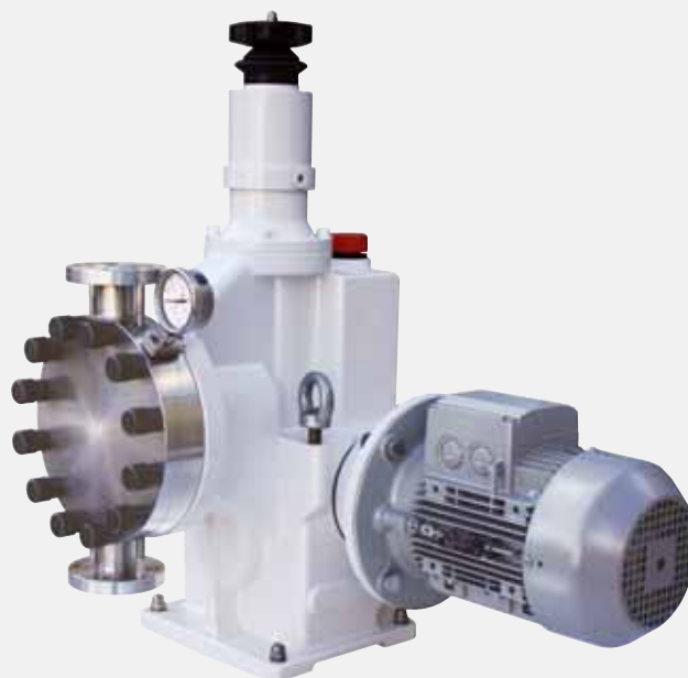
XL pump with single diaphragm and PVDF wetted parts. Automatic adjustment of the flow rate via OBL-designed electrical actuator that being IP66 and thanks to the anticondensation heater, turns out to be suitable for installation in harsh environments such as saline and/or deserts areas with high humidity and wide temperature variation.
