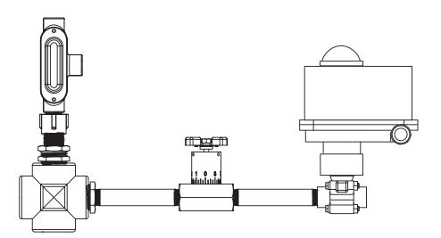
AVP valve packages take the guess work out of blowdown plumbing configurations. AVP's are factory pre-assembled to meet your boiler application pressure requirements complete with the probe cross (probe not included) and correct pipe lengths between components. Make installations even easier using prefabricated option P and we will pre-wire and mount your controller.
