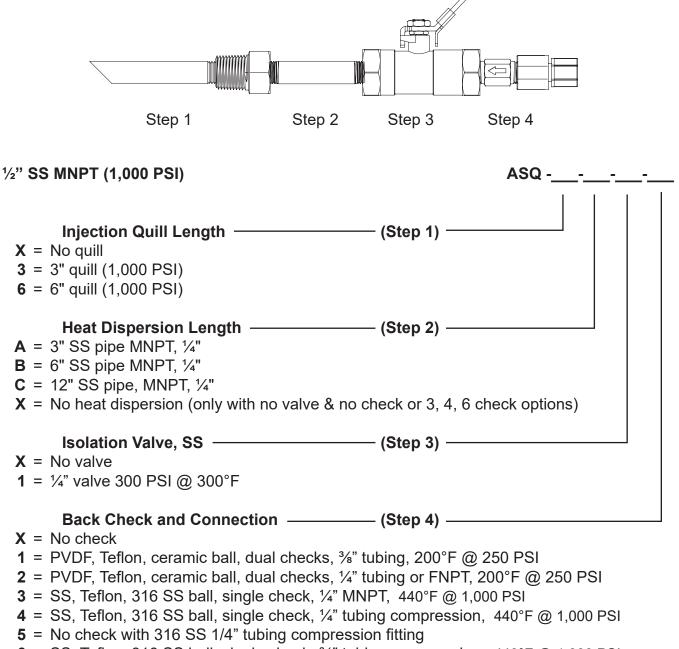
6 = SS, Teflon, 316 SS ball, single check, <sup>3</sup>/<sub>4</sub>" tubing compression, 440°F @ 1,000 PSI
