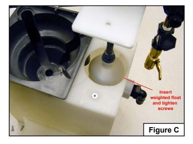
**WARNING:** Transporting the feeder with the weighted float attached to the hanger can damage the hanger and cause the valve to not shut-off correctly.
