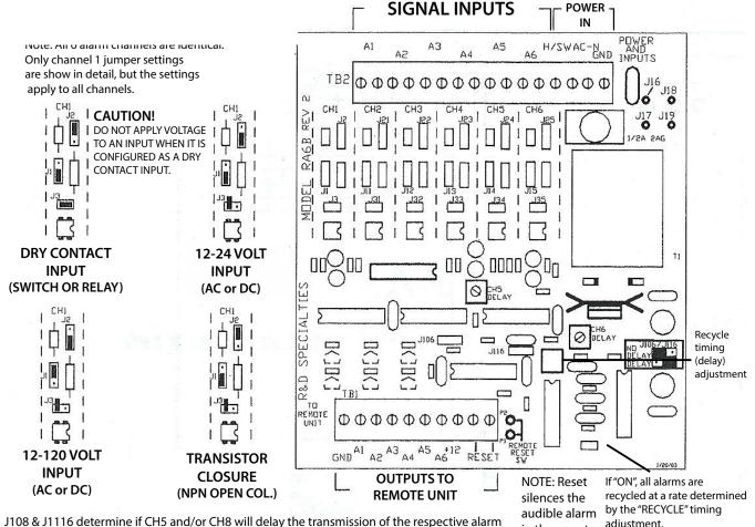
signals to the remote. If either delay is selected, it's timing (delay) is adjustable as follows: CH5 -- 15-30 sec.
