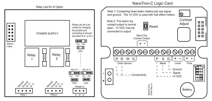
Note: Relay 1 is for drain alarm. Relay 2 is for Flush Timer
