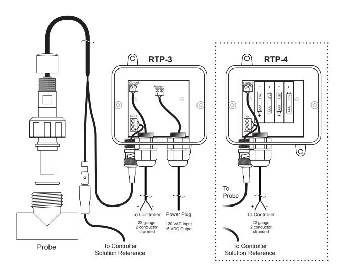
Pre-amps are supplied with both a BNC or two-conductor wire cable to connect between pre-amp and controller. The two-conductor cable can be ran directly to the pH input on the controller board. The BNC connector requires a special extension cable.
